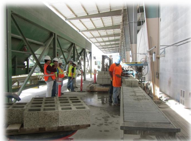
Burnished CMU blocks in production
